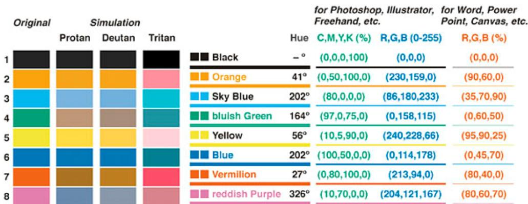
Fig. 16 Colorblind barrier-free color pallet
